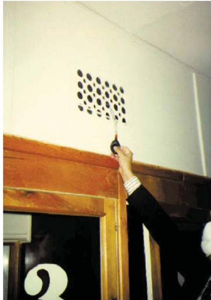
Using a smoke tube to monitor air flow in sputum collection booth at a TB facility in Riga, Latvia
